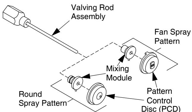
**FIG. 3: Mixing Module & PCD**
