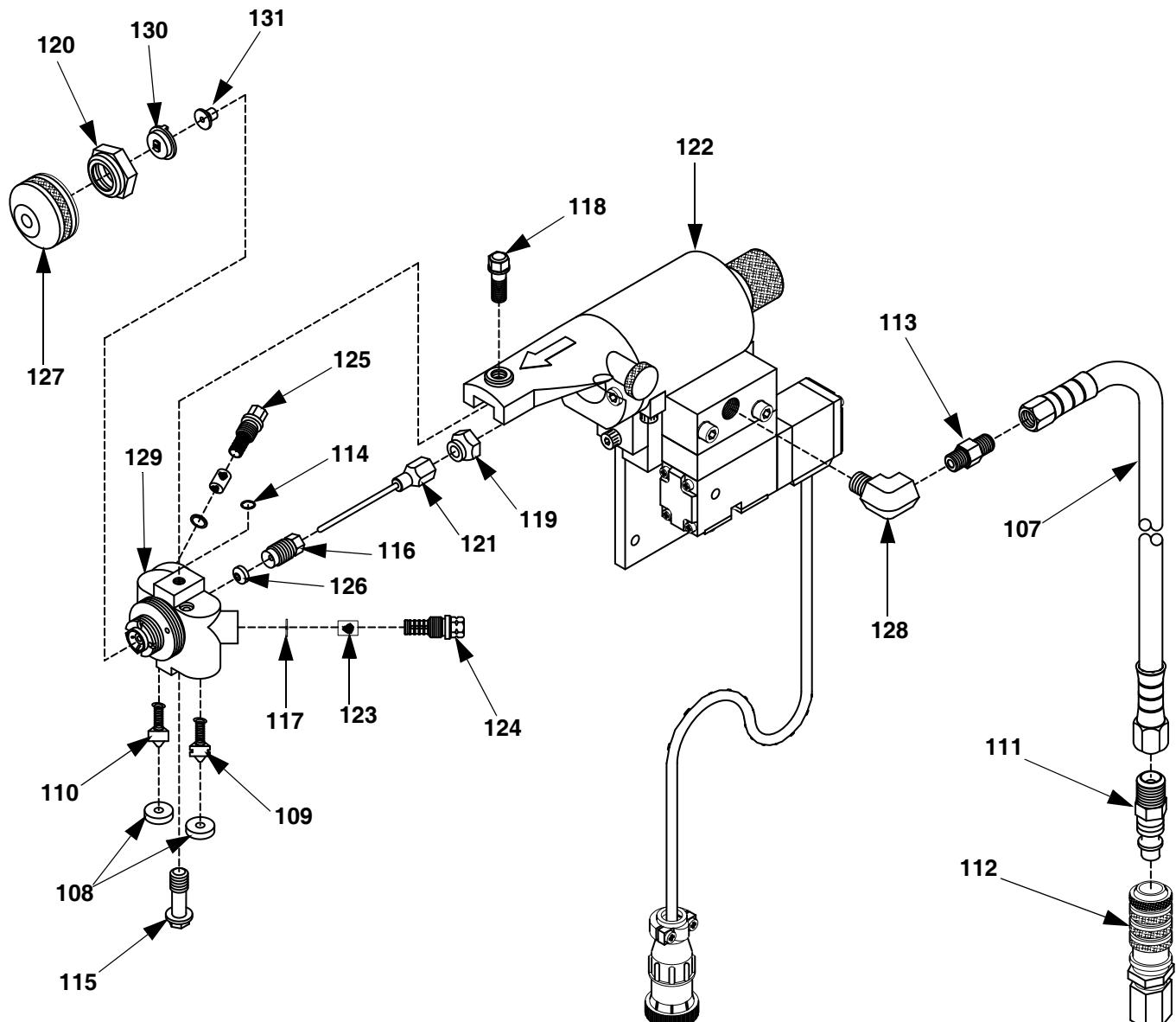
FIG. 21: GX-8P Spray Gun Final Assembly
