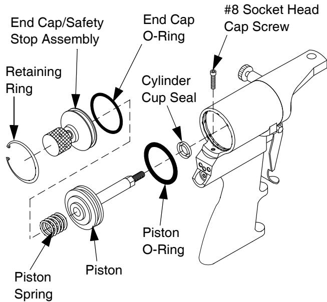
**FIG. 16: End Cap and Air Piston Assembly**
