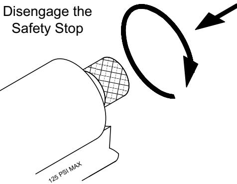
FIG. 5: Safety Stop - Disengaged
