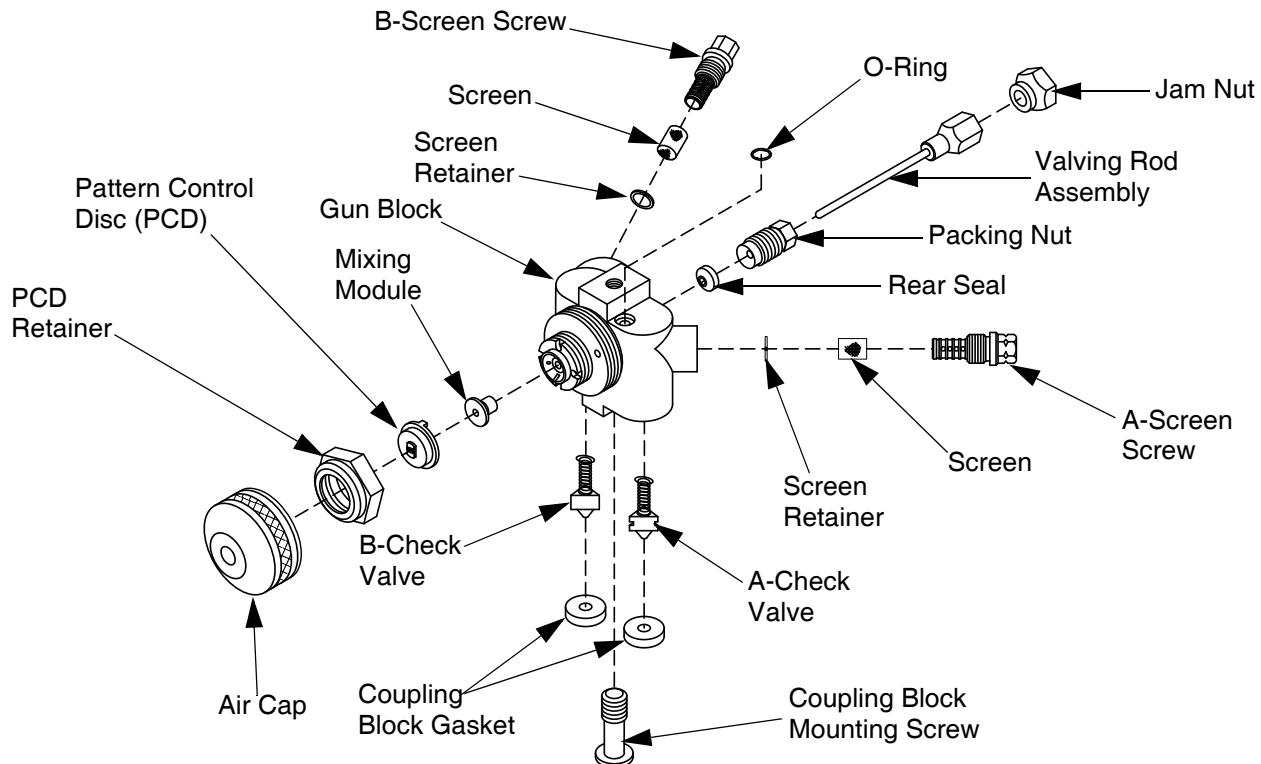
FIG. 2: GX-8P Centerline Components
