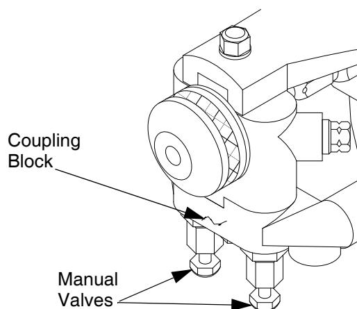
FIG. 7: Open Manual Valves
