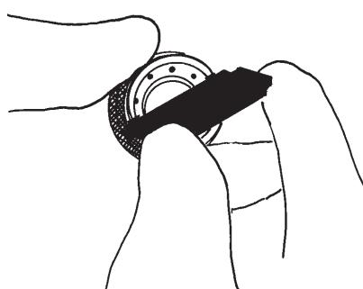
**FIG. 19: Untread Cap from PCD Body**
