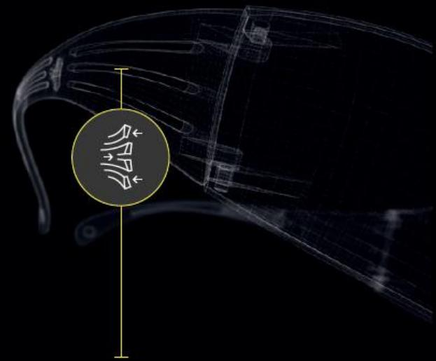
The diagram shows a side view of the temple of the safety glasses. A circular callout on the temple contains a detailed illustration of the 3M pressure diffusion technology, showing a series of vertical ridges with small gaps between them. Arrows point to these gaps, indicating the direction of pressure diffusion.
