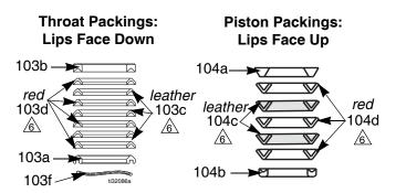
Lubricate Packings (soak leather packings in oil for 1 hour)
