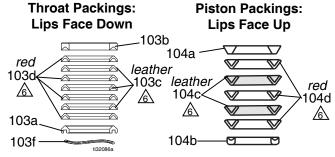
Lubricate Packings (soak leather packings in oil for 1 hour)
