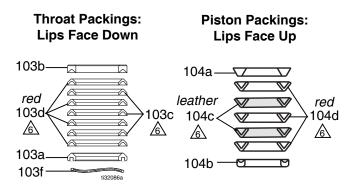
Lubricate Packings (soak leather packings in oil for 1 hour)
