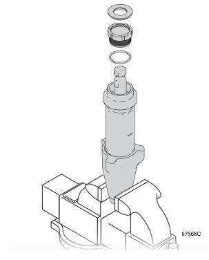
2. Unscrew intake valve from cylinder.
