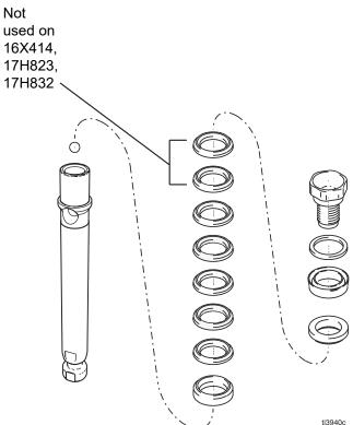
Remove throat packings and glands from cylinder. Discard throat packings and glands.
