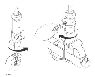
13. Torque packing nut (202) as follows:
