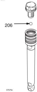
3. Tighten piston valve to piston rod as specified:
