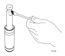
9. Grease o-rings (221 and 234) and place on sleeve. Slide sleeve/piston rod assembly into bottom of cylinder. Replace o-ring (207) if desired.
