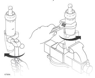
Disassemble intake valve. Clean and inspect o-ring (227). NOTE: A pick may be required to remove o-ring.
