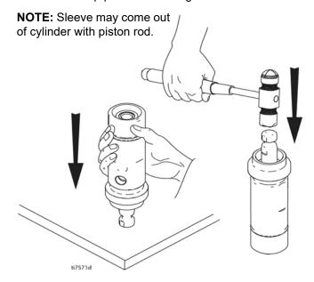
Remove piston rod from sleeve, or remove sleeve from cylinder. Mark IV and Mark VII models: Remove sleeve spacer (232) from sleeve.
