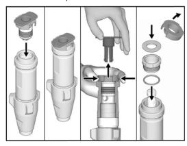
5. Install seal (201) into packing nut (202). Install o-ring (228) onto packing nut. Loosely install packing nut into cylinder.
