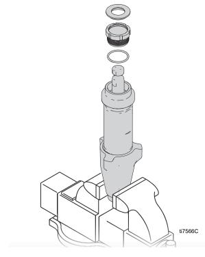
2. Unscrew intake valve from cylinder.
