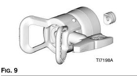
Screw the RAC tip assembly onto the gun and tighten firmly by hand.
