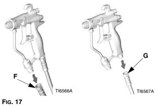
4. Connect the solvent supply hose (T) to the gun.
