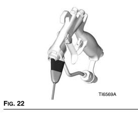
12. Scrub the air cap retaining ring (6), air cap (21), diffuser (5), and spray tip (33) with the soft-bristle brush. To clean out air cap holes, use a soft tool, such as a toothpick, to avoid damaging critical surfaces. Blow air through the spray tip to ensure the orifice is clean. Clean the air cap and spray tip daily, minimum. Some applications require more frequent cleaning.
