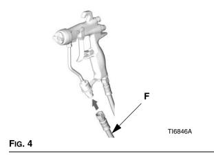
3. Connect the other end of the fluid hose (F) to the pump fluid outlet.
