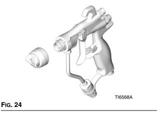
15. Dampen a soft cloth with solvent and wring-out the excess. Point the gun down and wipe off the outside of the gun.
