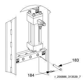
FIG. 4: Remove Pump Pins
