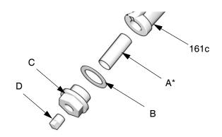
Fig. 15. Y Strainer Components
