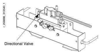
FIG. 2: Hydraulic Directional Valve Assembly
