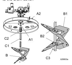
2. Tighten the lock nuts to 30 ft-lb (40.6 N·m).
