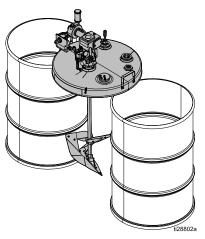
Install the four lock nuts (A2) holding the agitator to the drum cover.
