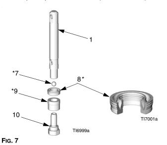
2. Lubricate piston u-cup (8\*). Push piston assembly into bottom of cylinder (6). Drive in with a non-sparking hammer
