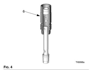
7. Using a 3/4 in. deep well socket, unscrew piston (10) from rod (1). Remove ball (7), u-cup (8), and bushing (9). See Fig. 5.
